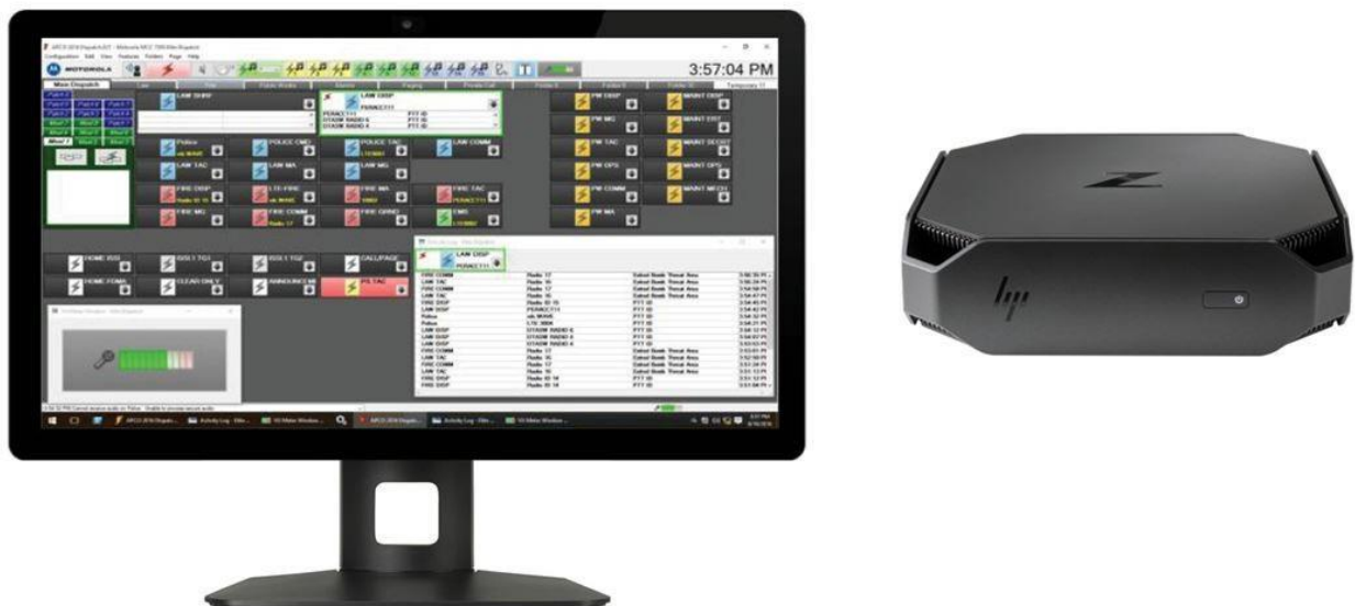
Figure 1-1: MCC 7500E Dispatch Position
