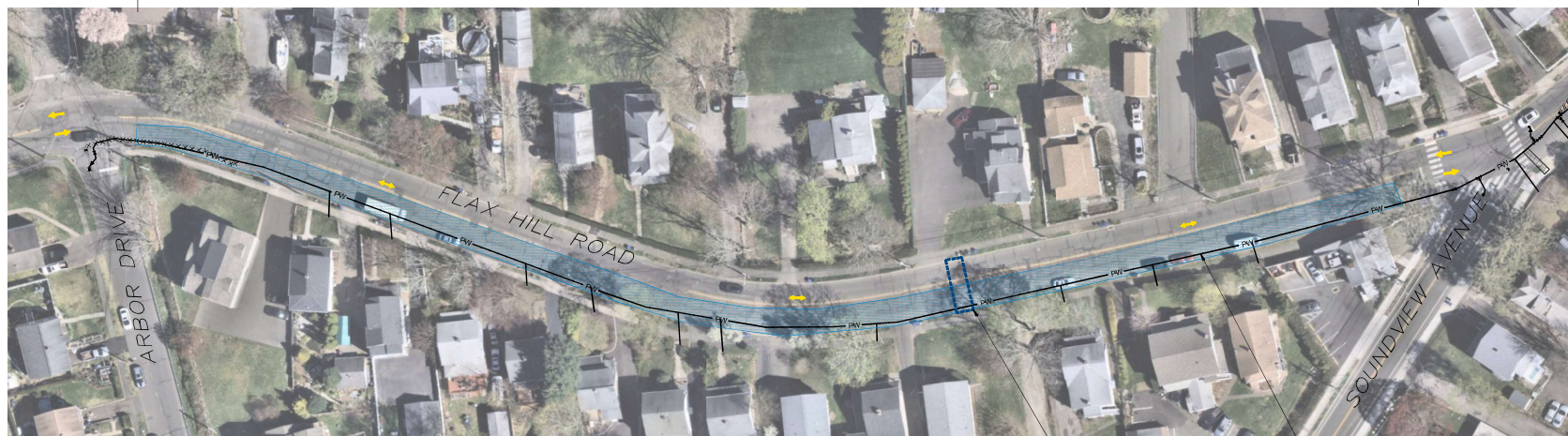
FLAX HILL ROAD TRAFFIC CONTROL PLAN PHASE B (MON-FRI, 7AM - 4PM)
