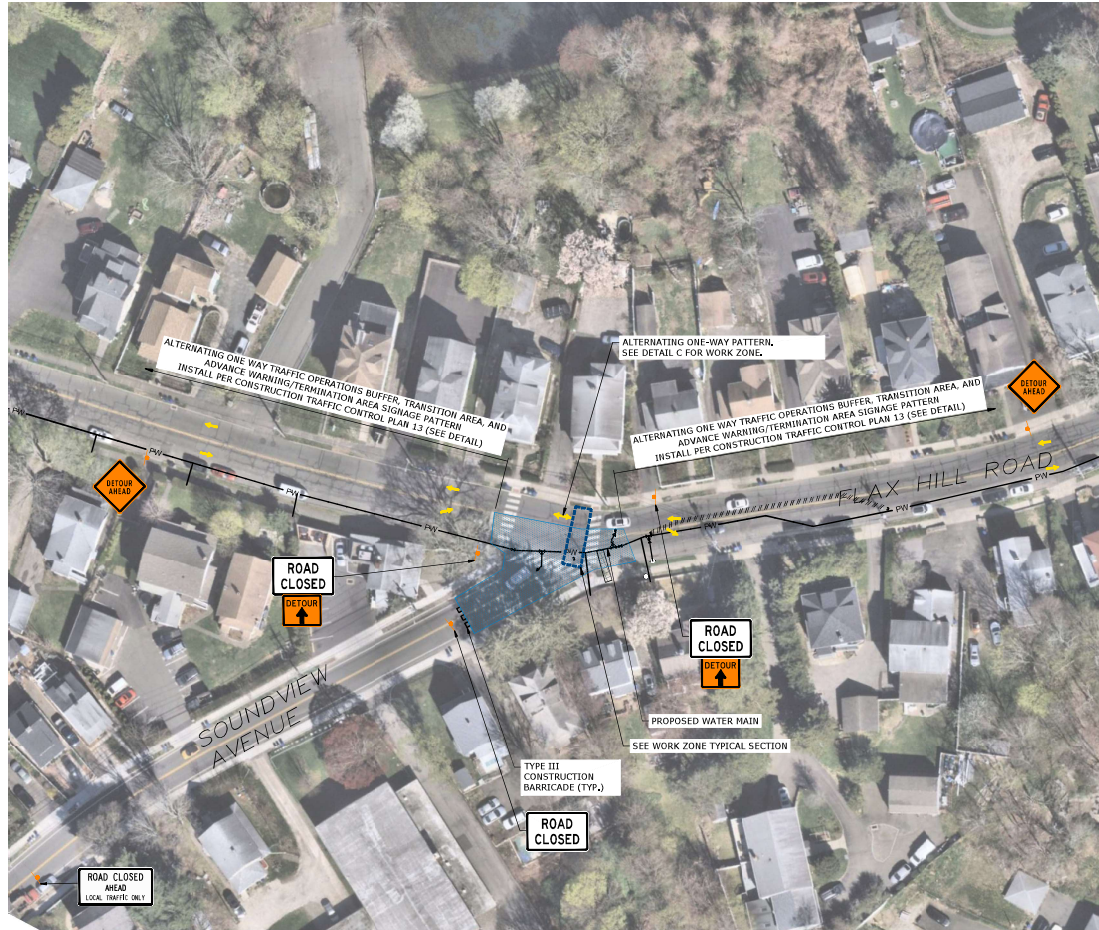
FLAX HILL ROAD - TRAFFIC CONTROL PLAN - PHASE C (MON-FRI, 7AM - 4PM)
