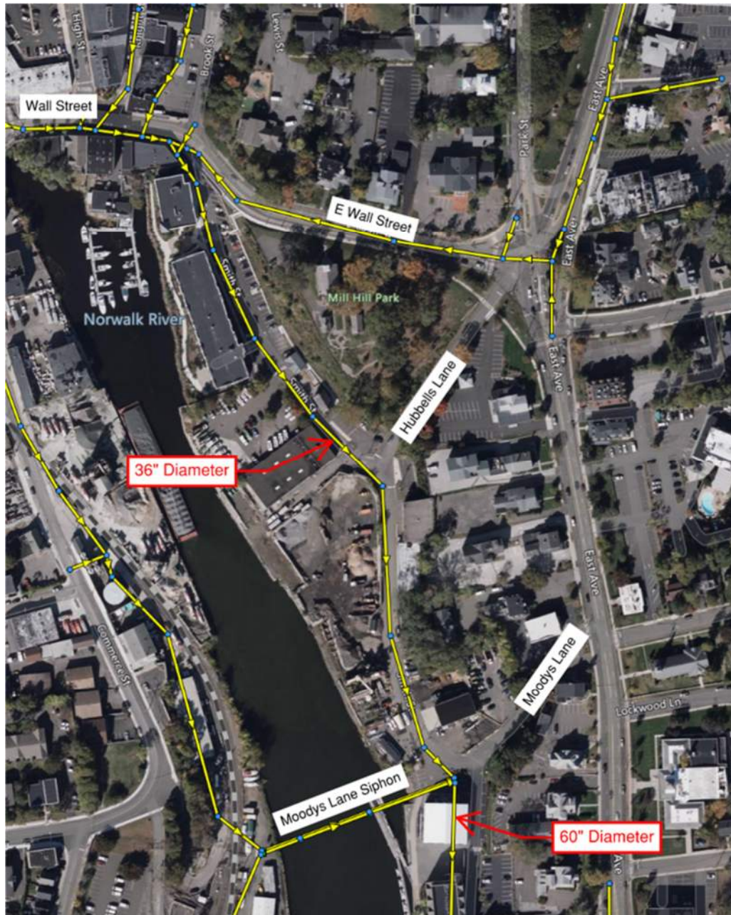
Figure 5-1. Sewer Layout Near Hubbells Lane
