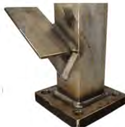
CLEANING GRADE "C"
