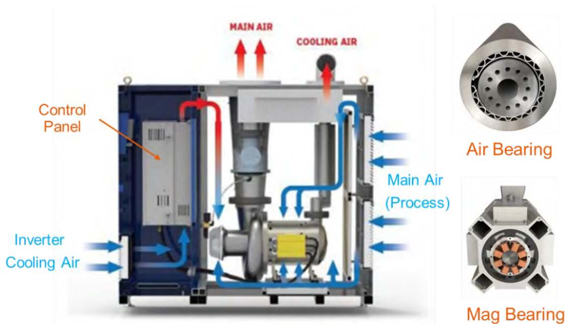
Figure 3. Typical Turbo Blowers Layout (LPR Global)
