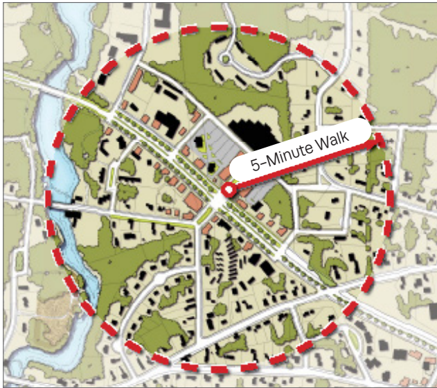
ILLUSTRATION 5.1.4.B-2 LINEAR PEDESTRIAN SHED
