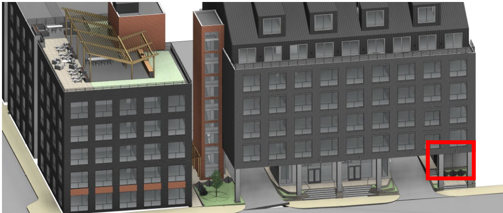
Figure 3: Trash Room from Aerial View
