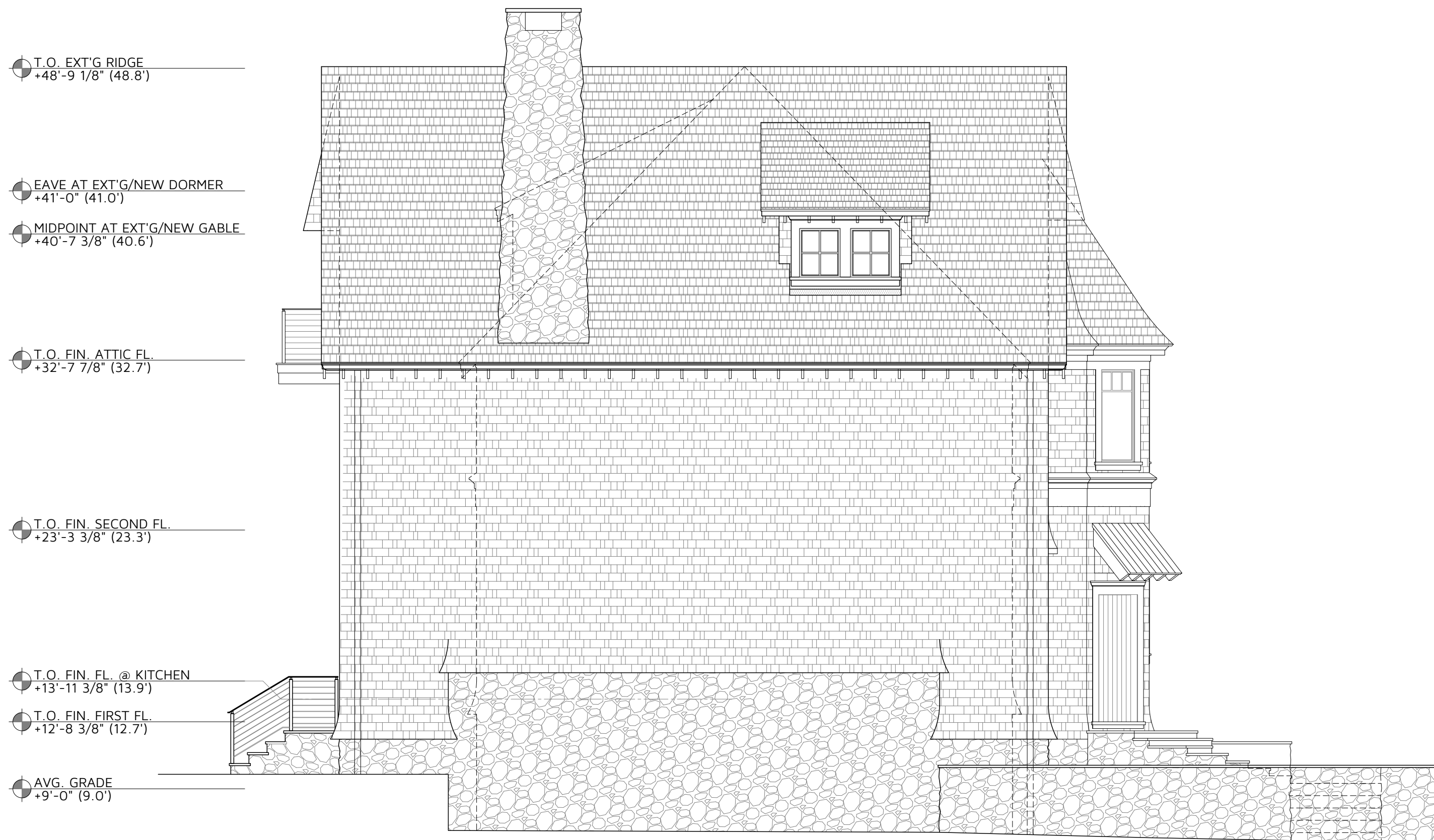
EXISTING LEFT ELEVATION (SOUTH) SCALE: 3/16" = 1'-0"
