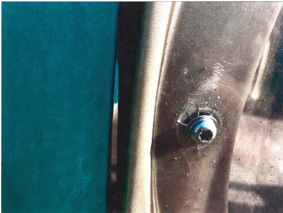
Priority 5 Safety Concern: Cracking on bubble panel plastic
