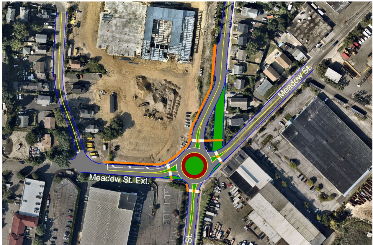
Figure 3. Proposed Roundabout Concept Plan – Aerial Image Background
