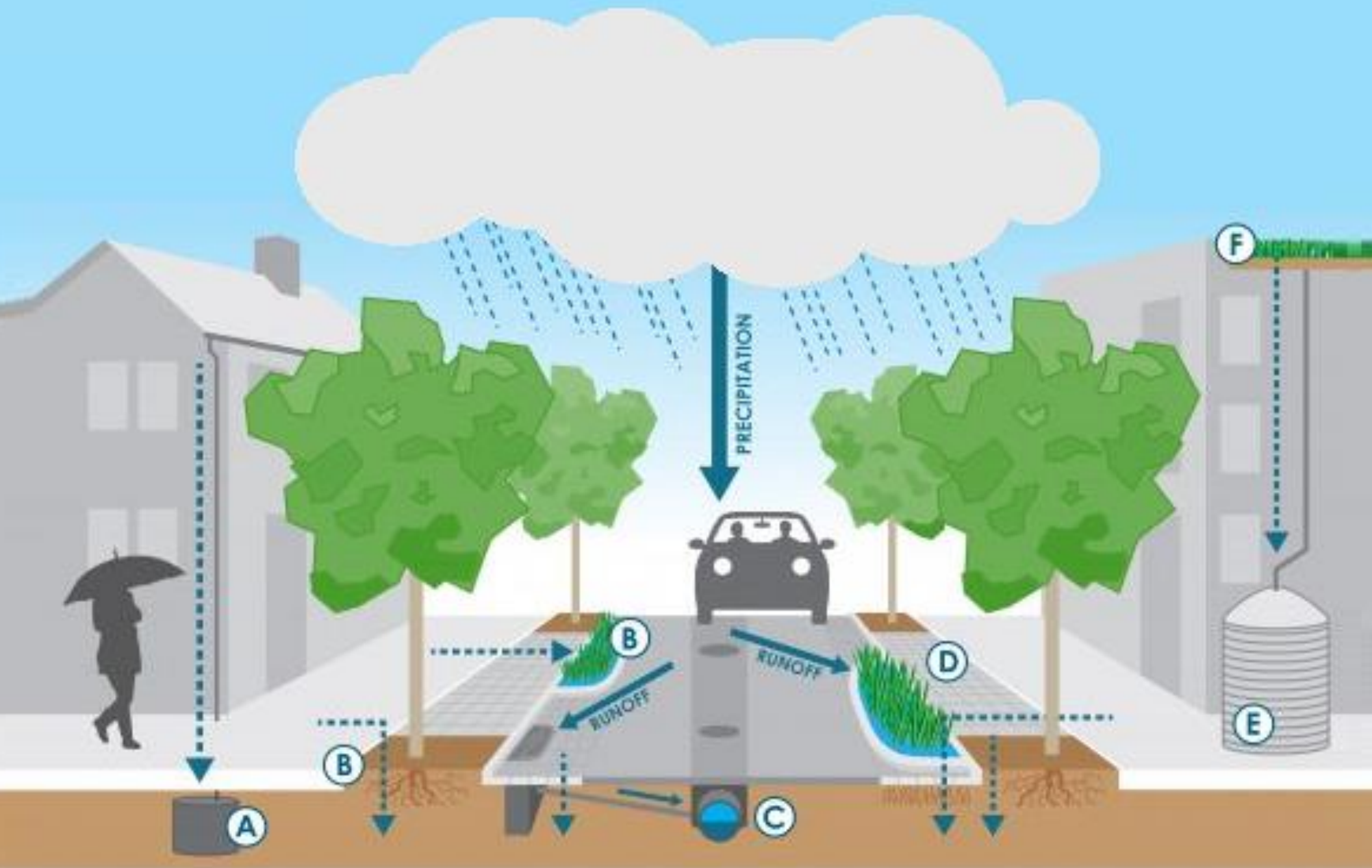
A: Dry Well B: Stormwater Planter C: Storm Drain D: Permeable Paving E: Rainwater Harvesting Cistern F: Green Roof
