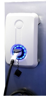
EV charger without a display screen, showing a lighted indicator. In addition to the color, charging progress might be indicated by the number of LEDs illuminated. Section 508 requires auditory or tactile indication in addition to visual cues.
